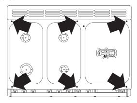
Taking care not to damage the burner electrodes, carefully lift the hotplate, from underneath disconnect the earth lead at the right hand rear from the rear cross member and withdraw the hotplate.
